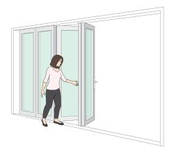
Close the next set of folding door pairs, using the recessed handle on the edge of the door to pull them closed.
