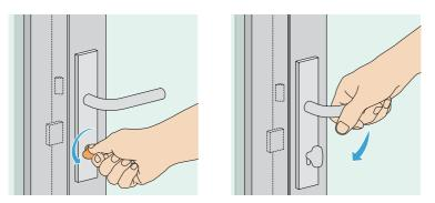
2. Unlock the door by pushing the handle downwards. This retracts the auxiliary bolts and also retracts the door latch.
