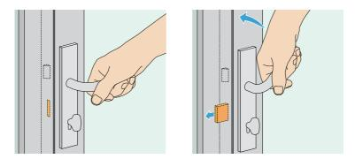
Lock the mechanism by rotating the thumbturn or key through 360°. (Note the thumbturn or key will only turn in one direction). When locked, the lever can no longer be operated from either inside or outside – check this by attempting to open the door.
