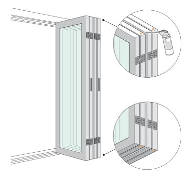
6. Door handles and key cylinders. Use a PTFE based dry lubricant spray. Teflon by DuPont® is one well-known trademark for PTFE. For key cylinders, use an extension nozzle, spray lightly into the keyway, then insert and remove the key 10 times to disperse the lubricant inside the cylinder before it dries.
