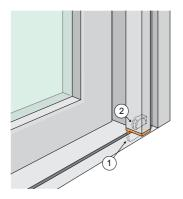
Autolatch<sup>™</sup> bolts at the top and bottom of locking locations. These are located at the top and bottom of the panels which house the hidden handle.
