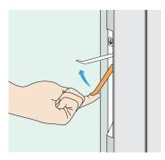
If you have a keyed AutoLatch<sup>™</sup>, then additionally you can key lock the doors. The key cylinder is concealed in the edge of the stile near the glass, and the locking operation is a 45° turn of the key which creates a distinct click, and when locked the lever can no longer be operated.
